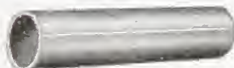
No. SF 755 STAINLESS STEEL BEER PIPE \frac{5}{8} in. outside diam. \times 21 g. plug drawn inside, polished outside.
